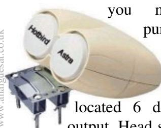
LNB known as 'Monoblock'. This LNB has two heads that are located 6 degrees apart, and a single output. Head selection is made through use of an integrated DiSEqC switch (see below for an explanation of DiSEqC). Some Monoblocks are self-contained, while others are incorporated into a bracket that attaches directly to the dish. You can also get dual-output Monoblocks which provide independent selection of both heads by two receivers.
