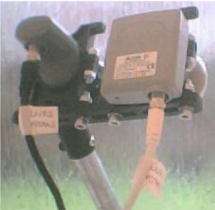
Connect the LNB and receiver cables to the DiSEqC switch and place the waterproof cover over it. Mount the switch at your chosen location.
