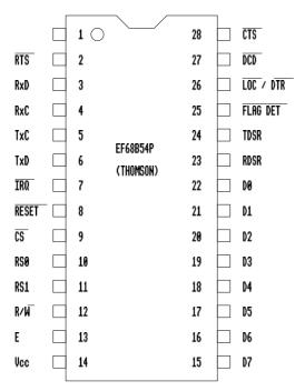
Econet operates by linking Econet almost as a fifth podule. The data is linked to the DB0-DB7 on the data bus. It uses LA2 and LA3 of the address bus (similar to the serial controller and floppy controller). The remaining parts (read/write, Econet FIQ etc) link into the IOC.
