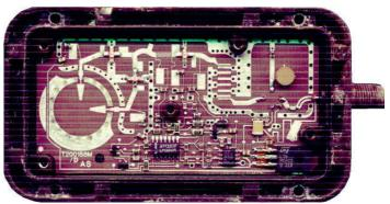
The picture above is from an old single-band LNB from the early days of Sky television. *NEVER OPEN UP AN LNB THAT YOU WISH TO USE*, treat them like harddiscs – keep 'em sealed! The "antenna" is the part on the left. The feed horn concentrates the signal to the two arrows. One arrow is for horizontal, the other for vertical. Exactly how it works is a careful blend of science and magic.
