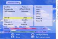
be ignored) and then the appropriate DiSEqC input. In this example I have selected "Astra 1" as the satellite and 'LNB1" as the input. The setting is saved, and the procedure repeated for the other satellites.
